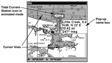
Navionics chart showing Tidal Current Station icon selected by cursor. In this example, the tidal current is in flood but it's about to enter the slack water stage. The current is flowing to the west at  $0.1 \, \mathrm{mph}$ .
